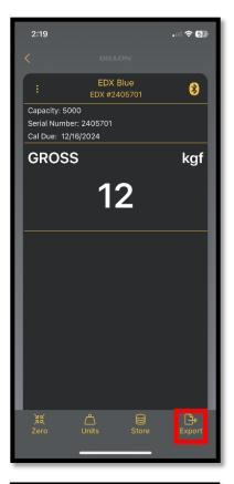
This will take users to a screen with the stored data page with the option to export as a PDF or Excel file. The logs will contain stored force readings with units and time stamps, as well as noting the unit's serial number, capacity, and calibration due date. Users can export the information in any format supported by the mobile device (email, airdrop, iMessage, text message, etc.)
